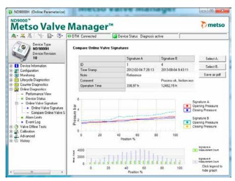
Valve Online Signature feature shows friction of the control valve online, under normal process conditions when ever the valve is changing position.
