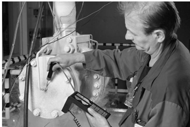
L6 is an excellent valve for cryogenic applications, temperatures -200 ... -46 °C / -320 ... -50 °F. Tight sealing over a wide range of cryogenic temperatures is accomplished with a high nickel alloy seat which maintains its mechanical properties even at cryogenic temperatures. The testing of the cryogenic valves is done in the Metso cryogenic laboratory in Finland. The testing procedure is agreed together with customer to fulfill the available standards and requirements.
