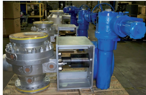
Figure 2. Metso MBV coke drum isolation valve
