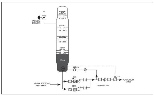
Fig 1. Principal PI drawing of an atmospheric distillation tower vacuum breaker.
