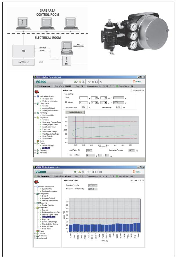
Fig 2. Neles ValvGuard tests the valve operation with partial stroke testing and these tests can be run automatically according to predefinied time interval. Each test is analysed and test results are stored into the device memory. With the trending feature user is able to compare latest test results and see how valve dynamics has developed during the lifecycle of device.
